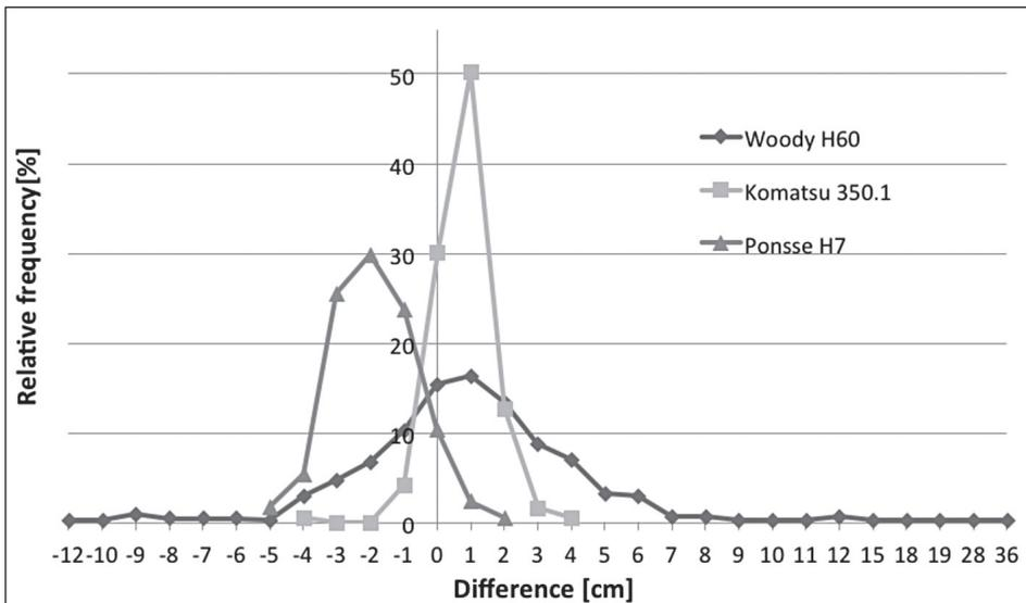
Figure 4: Log length differences of surveyed heads between reference method and machine's measurement in the state 'as is'.
