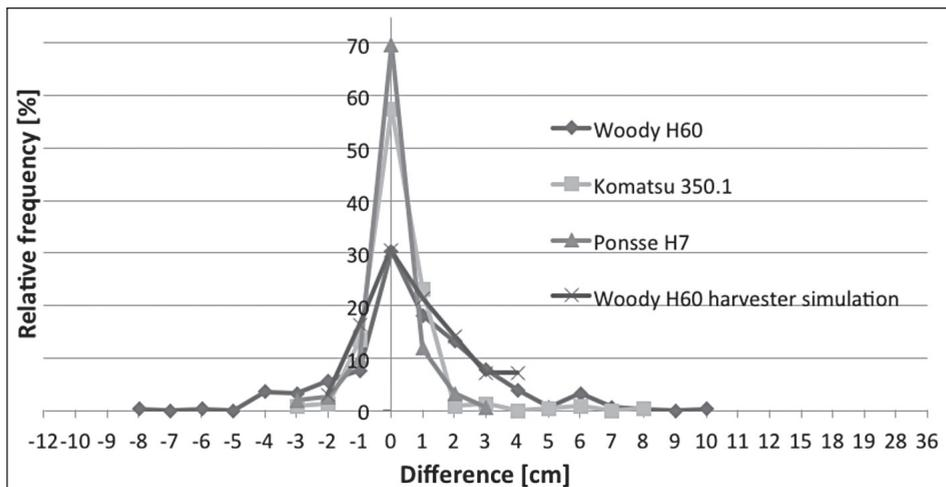
Figure 5: Differences of surveyed heads between reference method and machine's measurement in the state 'calibrated' and harvester simulation.
