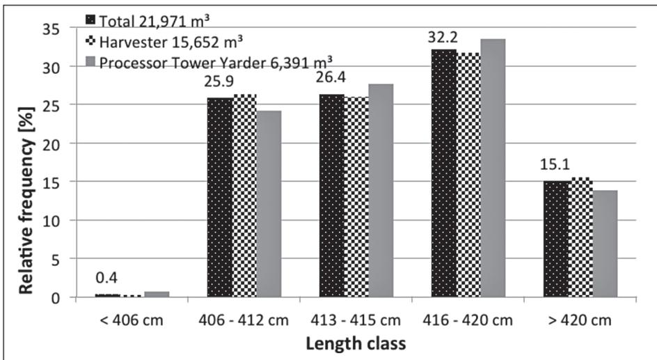
Figure 1: Distribution of laser scanned log lengths (at sawmill) separated by head type.
