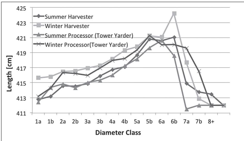
Figure 2: Log length depending on Diameter Class separated by head type and season.
