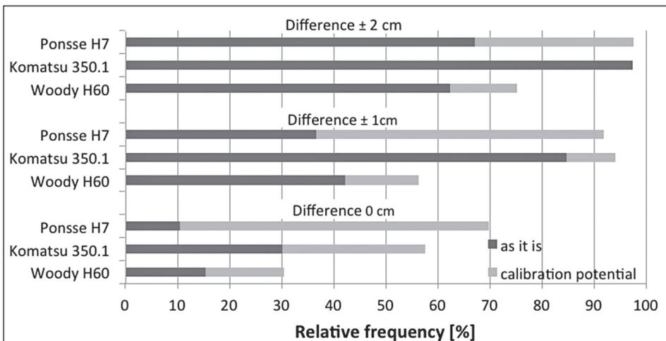
Figure 6: Professional calibration potential of the surveyed heads, swing the improvement through maintenance, calibration and professional advice.
