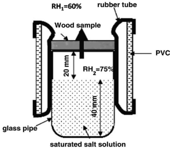
Fig. 2. Schematic of the experimental device (vapometer) used for measuring the diffusion coefficient (Tarmian et al. 2012)
