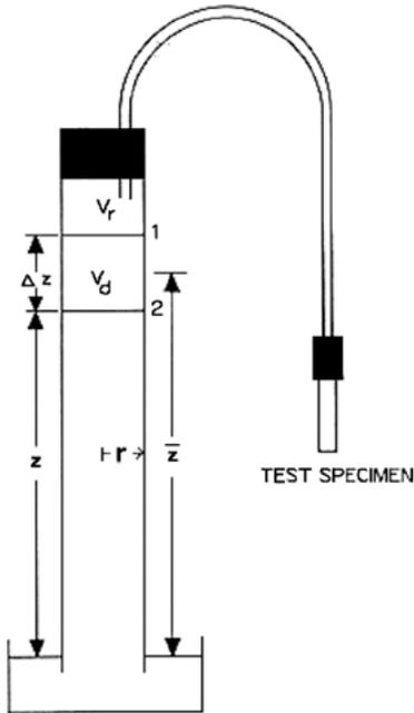
Fig. 1. Schematic view of the air permeability measurement apparatus (USPTO No. 8,079,249 B2) (Taghiyari, 2012 & 2013ab; Dashti et al., 2012a,b)
