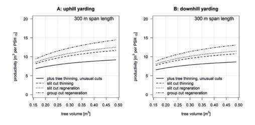
Figure 1: Productivity of a yarding with a Koller K507 dependent on tree volume, yarding direction and silvicultural treatment at a span length of 300 m.
