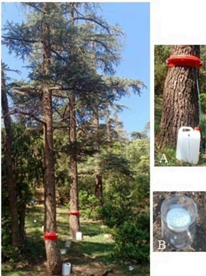
Figure 2: Devices for collecting stemflow (A) and throughfall (B).
